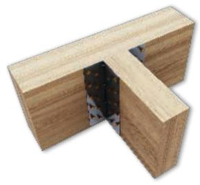
ECKO Split Hanger is made from 1.6mm G300 Z275 galvanised (internal use) steel to ensure it meets all requirements set out in NZS3604:2011 and have been BRANZ Tested to ensure structural performance.
