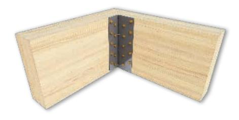
When installing a single split hanger additional end restraints are required. Use a minimum of 3 x M6 ECKO Construction screws or seek advice from project engineer. Screws should be aligned with centre of secondary beam and adhere to minimum edge from top/bottom of 50mm.
